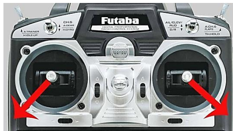
Figure 42 reset gyro to zero (example with Japanese Hand)
