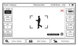
Watch Me/Follow Me Button: When in Smart Mode, press [6] to switch the TYPHOON between Watch Me and Follow me function. Follow Me function is the default setting, and the button is ORANGE. If it is GREY, it means ST10+ GPS isn't ready yet. Please wait.
