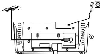
1. Insert the aerial cable plug into the AERIAL at the back of the TV-Video Combi.
