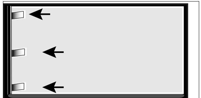
Step 1. WS-55515, WS-65515 and WS-65515A Diamond Shield molding clip removal
