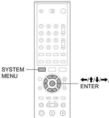
**1 Follow steps 1 to 4 of “Preparing for recording using the DV IN jack” (page 70), then press SYSTEM MENU.**
