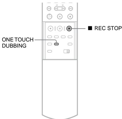
Follow steps 1 to 6 of “Preparing for recording using the DV IN jack” (page 70), and press ONE TOUCH DUBBING on the remote.
