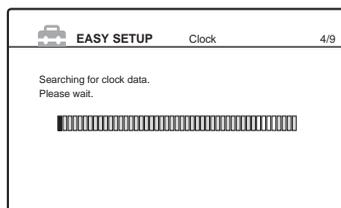
Once the clock signal is received, the Setup Display for selecting the aspect ratio of the connected TV appears.
