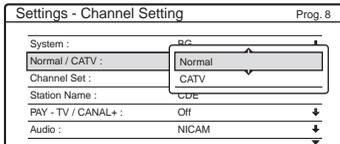
7 Select “Normal,” and press ENTER. To set CATV (Cable Television) channels, select “CATV.”
