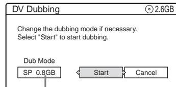
Data capacity required for the dubbing.
