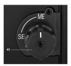
If no further exposure is desired with mirror lockup: Set multi-exposure knob **45** to "ME" (film advance disengaged) and trigger the camera with its lens capped. The reflex mirror will swing down again, and no frame will be lost. Then reset knob **45** to "SE".
