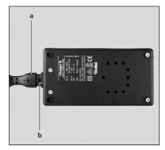
Place battery  $\boldsymbol{8}$  with its contacts onto the pins in the charger slot. Rapid charging will start after about 2 s, and the red LED glows. Cutoff voltage and battery temperature are monitored during charging. At the cutoff voltage, the unit switches to trickle charge. If the battery voltage exceeds the admissible maximum, the red LED will go out and rapid charging is interrupted until the temperature is back to normal.
