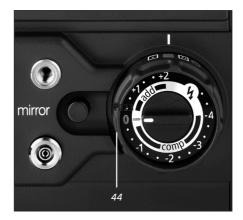
To select this mode, set dial **44** to ■. This icon will also appear in the display. To make allowance for special shooting conditions, multi-zone metering without center-weighting can be selected with switch **31** and the custom function "SF Cent" (see "Custom functions"). Centerweighting is then disabled as soon as switch **31** is turned on. The amount of center-weighting can be customized using MasterWare.
