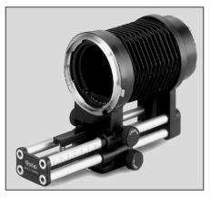
The **zoom extension tube** has a precise focusing mount and provides extensions from 22 mm to 68 mm. It thus covers the close-up range seamlessly, without changing individual components, and can be used in conjunction with the reverse adapter. It is suitable for use with any lens with a size VI filter bayonet.
