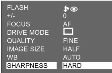
**3** Press the ▲ or ▼ toggle until the desired sharpness setting is highlighted.
