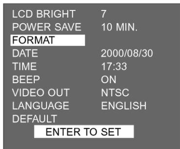
**3** Press the ▲ or ▼ toggle until [FORMAT] is highlighted, then press the ENTER button.
