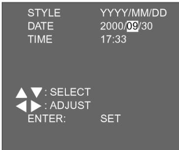
**7** Press the ▲ or ▼ toggle to set the date and hour. If you keep either of these toggles depressed, the setting will advance rapidly either forward or backward.
