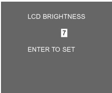
4 Press the ▲ or ▼ toggle until the desired brightness figure appears.
