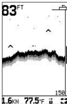
As the fish enters the weak edge of the sonar cone it generates a weak return signal that turns on the first pixel on the fishfinder screen. As the boat moves closer to the fish the distance between the transducer and the fish reduces and the return signal is displayed at progressively shallower depths, producing the start of an arch. When the fish is directly beneath the transducer and in the middle of
