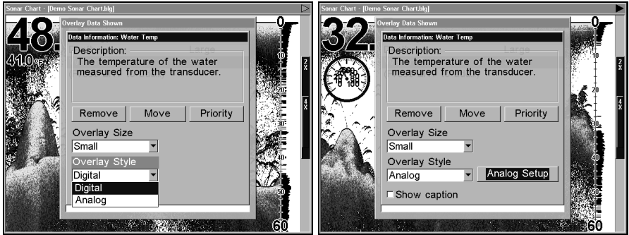
The Data Information menu (left) with Overlay style window activated. Choose analog and the Analog Setup button appears (right).
