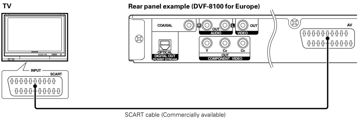
**Note** Make sure the DVD player is connected directly to the TV and not to a VCR, otherwise the DVD image could be distorted by the copy protection system.
