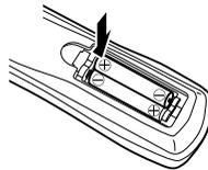
● Insert two R03 ("AAA"-size) batteries following the polarity indications.
