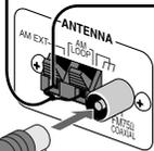
Disconnect the supplied FM antenna, and connect to an outdoor FM antenna using a 75  $\Omega$  wire with coaxial type connector (IEC or DIN45325).
