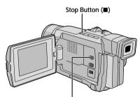
VIDEO/DSC Switch (GR-DVL910A/ DVL510A/DVL910EA/DVL510EA only; open the LCD monitor to access this switch)
