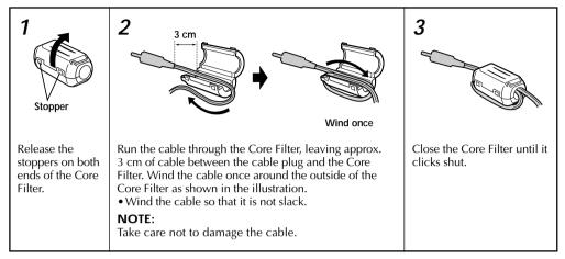
■ When connecting cables, attach the end with the Core Filter to the camcorder.
