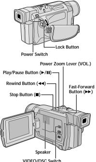
VIDEO/DSC Switch (GR-DVL910A/DVL510A/DVL910EA/ DVL510EA only; open the LCD monitor to access this switch)
