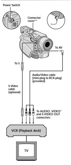
Connect when an S-Video cable is not used. \*\* When connecting the cables, open this cover. **Dubbing From A VCR**
