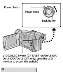
When the Power Switch is set to "▲", "▲" appears. When set to "∭" or " ☑ ", there is no indication.
