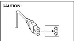
To avoid electric shock or damage to the unit, first firmly insert the small end of the power cord into the AC Adapter until it is no longer wobbly, and then plug the larger end of the power cord into an AC outlet.
