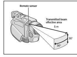
When using the remote control, be sure to point it at the remote sensor. The illustration shows the approximate transmitted beam effective area for indoor use.
