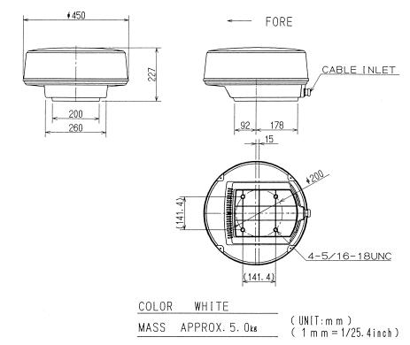
FIG. 3-4 SCANNER MOUNTING DIMENSIONS
