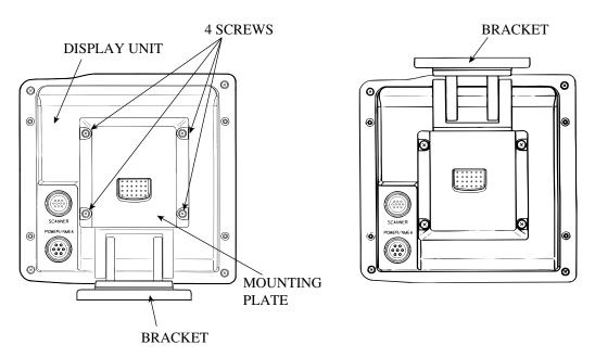
The display unit is separated from the bracket in the shipping carton. Install the display unit by sliding it onto the bracket until it is fully seated.
