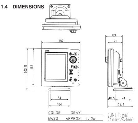
FIG. 1-1 DISPLAY MOUNTING DIMENSIONS
