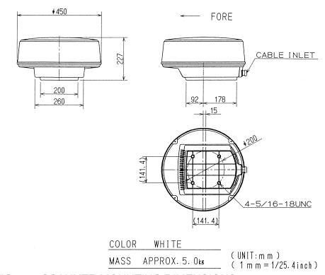
FIG. 1-2 SCANNER MOUNTING DIMENSIONS
