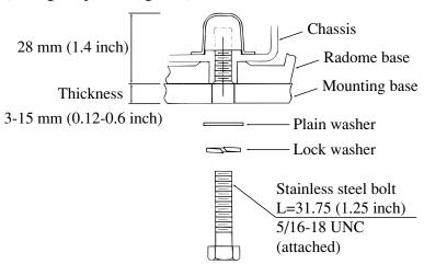
FIG. 3-5 MOUNTING BOLTS for SCANNER UNIT
