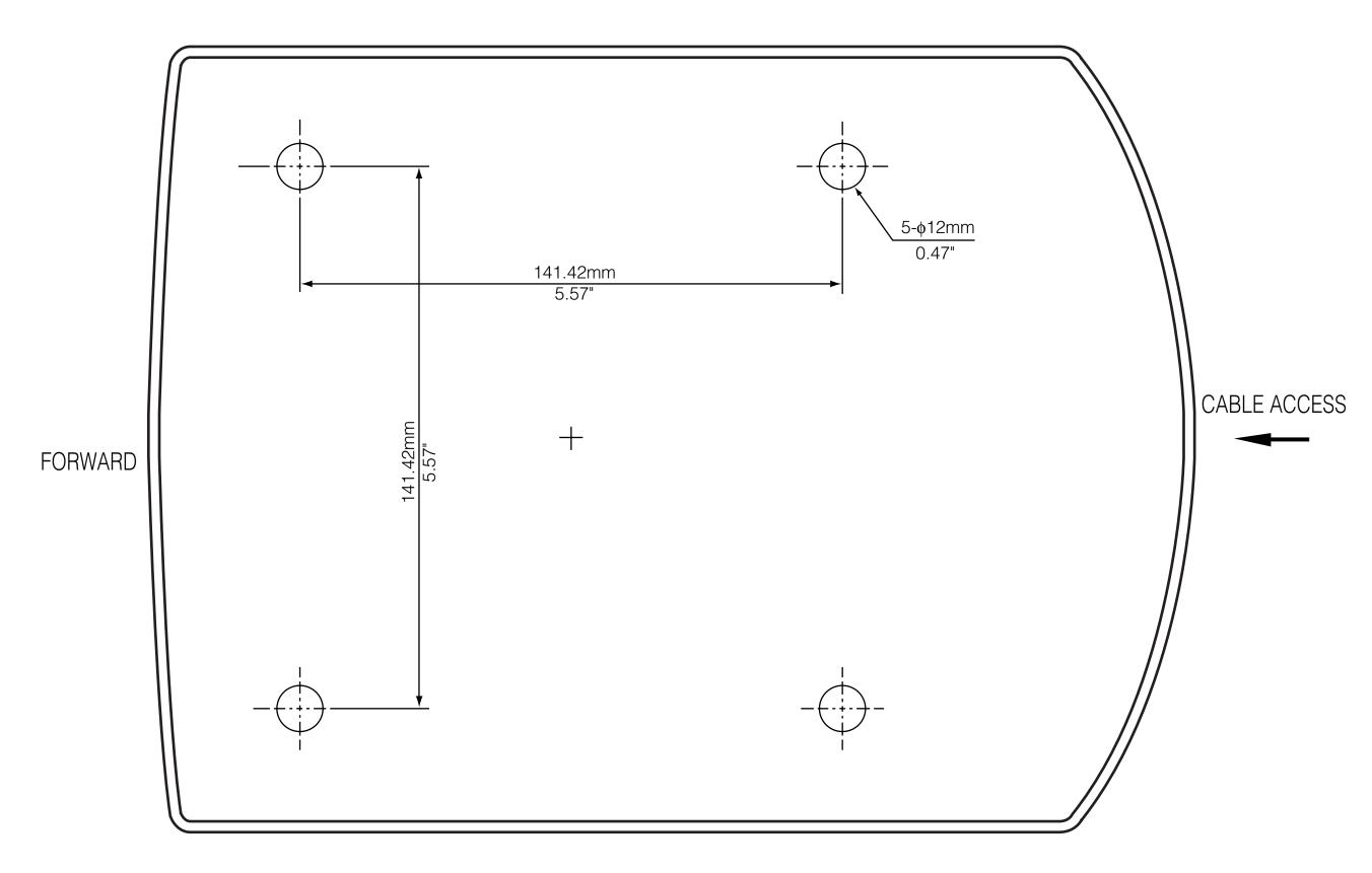
Fig.2 RADAR 1500 MK II SCANNER UNIT (NKE-1063) RADOME TEMPLATE
