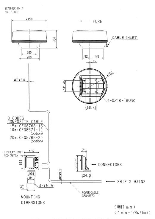
FIG. 3-1 GENERAL SYSTEM DIAGRAM
