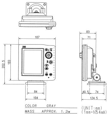
FIG. 3-3 DISPLAY MOUNTING DIMENSIONS
