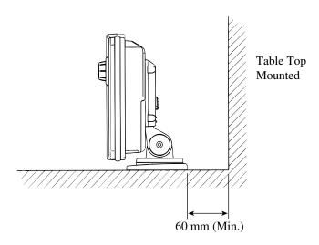
FIG. 3-2 TYPICAL MOUNTING METHOD
