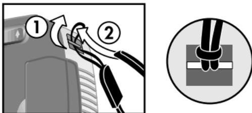
**NOTE** It is easiest to install the wrist strap by inserting it from the bottom of the camera.
