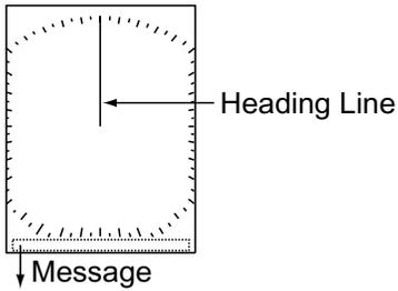
HEADING LINE ADJUSTMENT BY '←' AND '→' KEYS. THEN PUSH MODE KEY TO SET.
