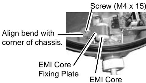
Align bend with corner of chassis.
