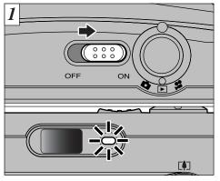
To switch the camera on and off, slide the power switch sideways. When you switch the camera on, the viewfinder lamp lights (green).
