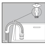
2. If necessary turn the unscrewing the nut at the Now tighten the nut anew to avoid leaks. (Open the does not leak and close it again.)
