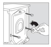
1. Unscrew and remove the three rear screws by means of a key.
