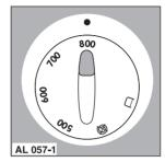
This dial allows the reduction of the final and the intermediate spin speed or to select NO SPIN or  $\boxminus$  RINSE HOLD options.
