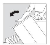
2. Lean the appliance back on the rear and fit one of the polystyrene angles between the appliance and the floor.
