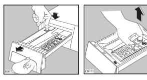
Detergent can also accumulate inside the drawer recess: clean it with an old toothbrush. Refit the drawer after cleaning.
