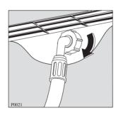
2. If necessary turn the hose adequately by unscrewing the nut at the rear of the appliance. Now tighten the nut anew to avoid leaks. (Open the tap and assure that it does not leak and close it again.)
