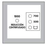
Press this button so many times as it was necesary until the relevant light turns on corresponding to the wished option.
