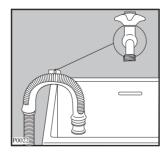
3. Place the discharging hose in a washbasin or sink with the aid of the bent piece delivered separately. The bent piece has to be entered into the tube's mouth in order to assure the support. Aforesaid piece allows the hose to be
