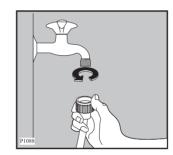
1. Carefully screw the pipe to the tap taking care not to damage the screwdrive and fix the nut well on to the end in order to avoid leaking.
