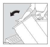
2. Lean the appliance back on the rear and fit one of the polystyrene angles between the appliance and the floor.
