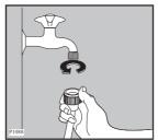
A) Carefully screw the pipe to the tap taking care not to damage the screwdrive and fix the nut well on to the end in order to avoid leaking.
