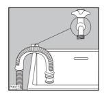
D) Place the discharging hose in a washbasin or sink with the aid of the bent piece delivered separately. The bent piece has to be entered into the tube's mouth in order to assure the support. Aforesaid piece allows the hose to be fixed to the wall by means of an opening on the upper part and that way the hose does not move and its falling is avoided.
