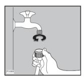
A) Carefully screw the pipe to the tap taking care not to damage the screwdrive and fix the nut well on to the end in order to avoid leaking.
