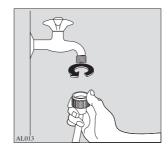
A) Carefully screw the pipe of the inlet hose to the tap taking care not to damage the screwdrive and fix the nut well on to the end in order to avoid leaking.
