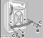
Remove the bracket **D** and tighten up the six smaller bolts **C**.
