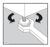
Any necessary adjustment can be made with a spanner. Accurate levelling prevents vibration, noise and displacement of the machine during operation. Some vibration is inevitable, especially if mounted on a
