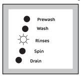
To select **Drain** the programme must be paused, now press the Skip button three times, the **wash - rinses - spin** LED,s go out.
