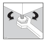
Any necessary adjustment can be made with a spanner. Accurate levelling prevents vibration, noise and displacement of the machine during operation.
