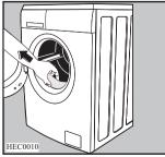
Fill the smaller upper hole and the two large ones with the corresponding plastic plug caps supplied in the bag containing the instruction booklet.
