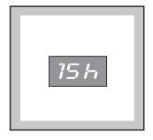
The delay time is displayed for 3 seconds, then the duration of the selected programme reappears.
