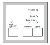
If you select the "Night Cycle" option, the machine will stop at the end of the programme with the water still in the tub.
