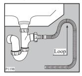
The drain hose may be extended to a maximum of 4 metres. An additional drain hose and joining piece is available from your local Service Force Centre. The joining piece must have an internal diameter of 18mm.
