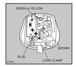
The wire coloured green and yellow must be connected to the terminal marked with the letter «E» or by the earth symbol  $\frac{1}{=}$  or coloured green and yellow.
