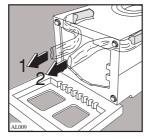
Place the machine in an upright position and remove the three plastic spacers.
