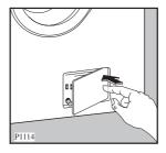
Place a container close to the pump to collect any spillage.  When no more water comes out, unscrew the pump cover and remove it. Always keep a cloth nearby to dry up spillage of water when removing the cover.
