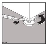
Any necessary adjustment can be made with a spanner. Accurate levelling prevents vibration, noise and displacement of the machine during operation.
