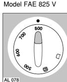
This dial allows the reduction of the final and the intermediate spin speed or to select **Ø NO SPIN** or **□ RINSE HOLD** (no-wrinkle) options.
