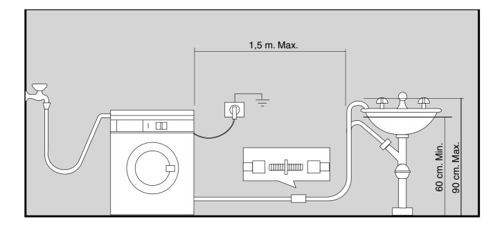
**IMPORTANT:** The distance from the floor to the highest part of the hose should be between 60 to 90 cm. (It is advised to be between 60 and 70 cm). The hose must not be bent nor twisted to avoid clogging. Should a prolongation of the discharging hose be unavoidable this must never surpass 1.5 m and must be of the same diameter as the original hose.
