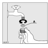
A) Place the enclosed rubber joint, delivered in a plastic bag together with the appliance (A) Fig.6), at the very end of the inlet hose and carefully screw the pipe to the tap taking care not to damage the screwdrive and fix the nut well on to the end in order to avoid leaking.
