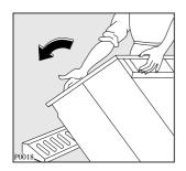
Lean the appliance back on the rear and fit one of the polystyrene angles between the appliance and the floor.
