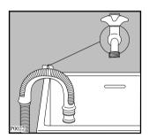
In a sink drain pipe branch. This branch must be above the tap so that the bend is at least 60 cm above the ground.
