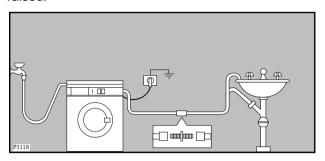
The drain hose may be extended to a maximum of 4 metres. An additional drain hose and joining piece is available from your local Service Centre.
