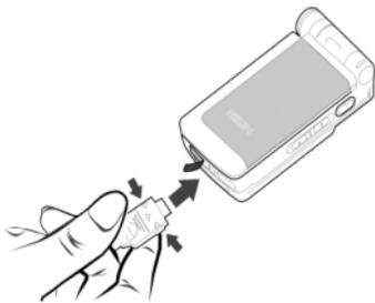
1. Once the battery and back cover is attached to the phone, plug the charger connector (supplied with the phone, in the box) into the charger socket at the base of the phone (arrow side up), and plug the other end of the charger to an easily accessible AC power socket.
