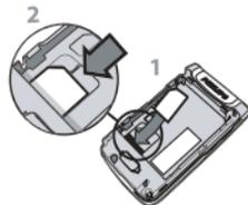
4. Insert the battery: first place its right side (connectors downwards) against the right edge of the phone and press until it clips.
