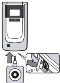
Connect the camera to display the camera preview screen: the lens of the camera is automatically focused and icons are displayed in the bottom: **Zoom**, **Effects**, **Camera mode**, **Shot**.
