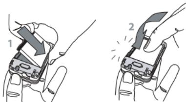
5. Replace the battery cover by sliding it into its slots, until it stops. Remove the protective film covering the screen before using the phone.
