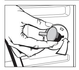
■ Close the holes with the rotary protectors, making sure to close the caps.
