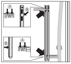
■ Fasten the shipping struts to the rear of the washer. Take care to insert the drill holes correctly, **(B)**, into the clamps, **(A)**.
