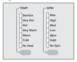
Press the "TEMP" and "SPIN" buttons until the indicator of the desired setting lights.
