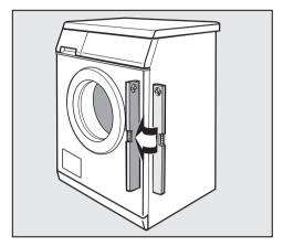
Failure to level the machine can result in increased water and energy consumption, loud noises during the spin cycle or "walking" across the floor during use.
