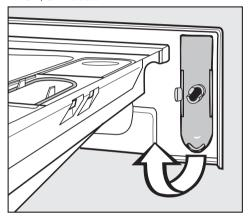
To clean the lint trap, remove the tool from behind the detergent dispenser drawer.
