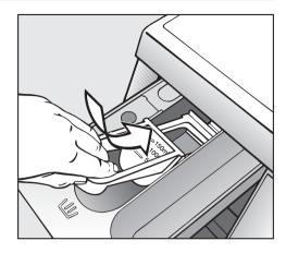
If you are washing with liquid detergent, use the liquid detergent insert in the main wash compartment ......
