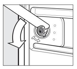
■ Turn the left shipping strut counterclockwise 90° with the enclosed combination wrench.
