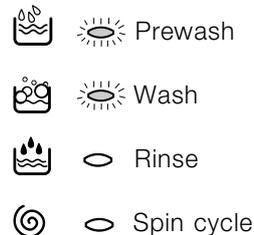
Note: during draining, the LED corresponding to the Spin cycle phase will be turned on.
