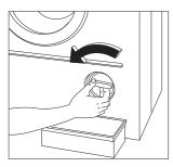
A clean filter is important for correct functioning of the washing machine, and it should therefore be cleaned regularly. Small objects left in the pockets and yarn ist retained here. Unscrew the filter completely turning it
