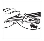
If it takes longer to fill up the washing machine it is time to check the water inlet hose filter it may be clogged. Turn off the water tap. Unscrew the fixing nut of the inlet hose. Remove the filter from the electrovalve and clean it with a hard bristle brush and replace it. Screw on the nut thoroughfully.
