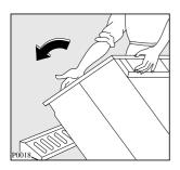
Lean the appliance back on the rear and fit one of the polystyrene angles between the appliance and the floor.
