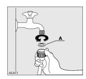
A) Place the enclosed rubber joint, delivered in a plastic bag together with the appliance (A) Fig.6), at the very end of the inlet hose and carefully screw the pipe to the tap taking care not to damage the screwdrive and fix the nut well on to the end in order to avoid leaking.
