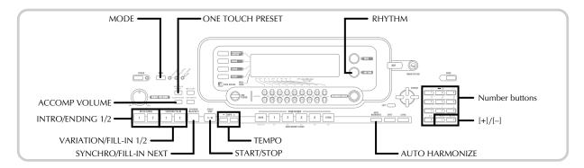
This keyboard automatically plays bass and chord parts in accordance with the chords you finger. The bass and chord parts are played using sounds and tones that are automatically selected to select the rhythm you are using. All of this means that you get full, realistic accompaniments for the melody notes you play with your right hand, creating the mood of a one-person ensemble.
