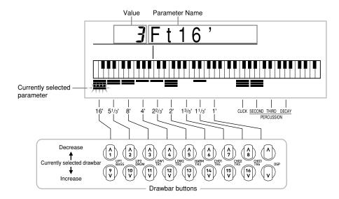
Each of the nine button pairs is assigned values ranging from 16 feet to 1 foot. Each button pair has a decrease button (for decreasing by 16 feet, 5-1/3 feet, etc.) and an increase button (for increasing by 16 feet, 5-1/3 feet, etc.).
