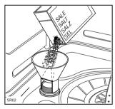
When this has been done, all that is then required is to periodically top up the container with salt. You are reminded of this by the Salt Refill Indicator Light  $\subseteq$  on the control panel which will illuminate when the salt has finished.
