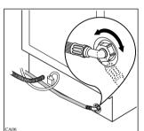
**Note:** the end of the hose connected to the machine can be positioned as required, by simply slackening the retaining ring.
