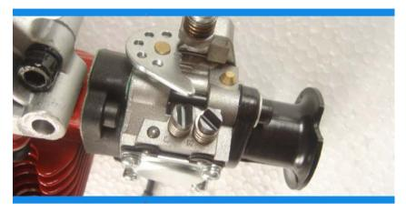
Before each engine is shipped it has to pass QC and is then test run. We do a basic adjustment of the carburetor needles at that point.
