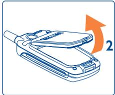
Lift up the battery and remove it
