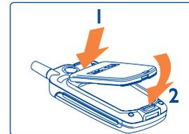
Align the tab on top of the battery to the slot in the battery compartment of your phone.
