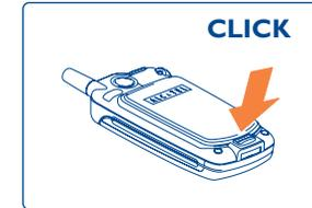
Press down the battery until the latch is completely locked.
