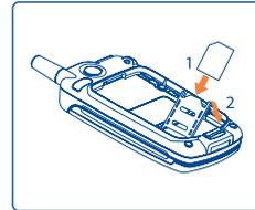
Before inserting the SIM card into the slot, push SIM card catch in the "OPEN" direction until it is released. Place the SIM card into the slot with care.
