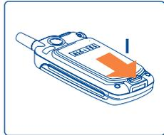
Press and hold down the latch in your phone. Push it outwards as shown until the battery is released.
