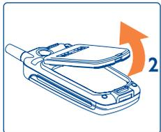
Lift up the battery and remove it
