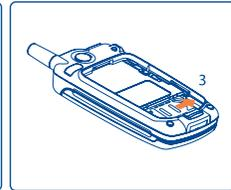
Make sure the cardnotch is on the upper right hand side. Press and hold down the catch and push it until it is locked.
