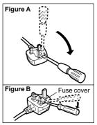
2. Replace the fuse and close or attach the fuse cover.
