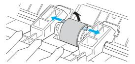
5 Gently pull the pickup roller up and out.
