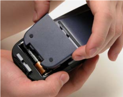
Replace battery compartment cover. Align tabs with slots in the base, left. Press latch firmly until it clicks, as shown right
