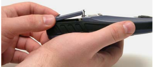
Remove Atlas battery cover.
