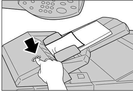
2. Open the cover 1e and then remove the jammed paper and all paper loaded in the Interposer.
