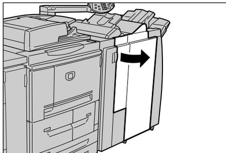
2. Pull out the tri-fold output tray 2d, swing lever 2g, and remove the jammed paper.
