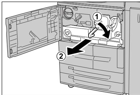
3. Lift up the lever 2b to remove the jammed paper. Turn the knob 2a to remove the jammed paper as necessary.
