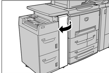
2. Open the lower left cover while gripping the release lever.
