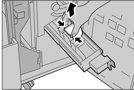
4. Remove the jammed staples as shown in the illustration.
