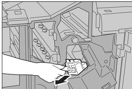
4. Push the positions indicated by arrows to remove the staple case from the cartridge.
