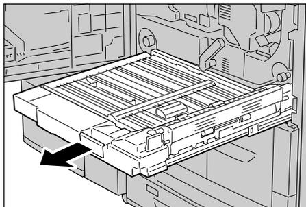
3. Move the release lever 3a to remove the jammed paper.
