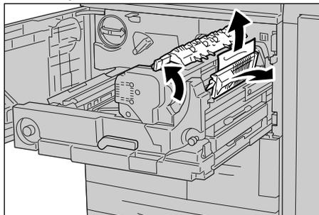
6. Turn the knob 2f as necessary and then remove the jammed paper.
