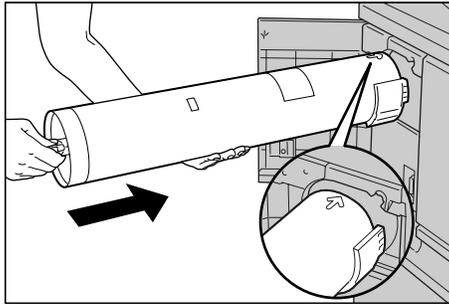
6. Push the toner cartridge slowly to the end and turn it to the right until it aligns with the lock sign.
