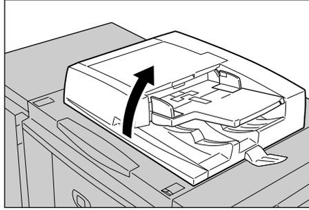
2. Open the belt area while gripping the lever and remove the jammed document.
