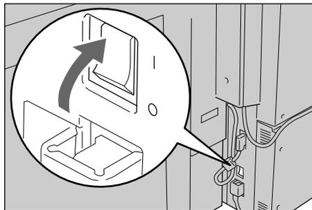
In the event of a current leakage, the breaker will automatically cut off the power circuit to prevent any leakage or fire from occurring.
