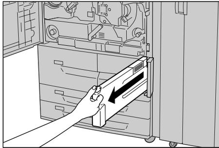
4. Hold the center part on the top of the bottle (as shown in the illustration), and then use both hands to remove the bottle.
