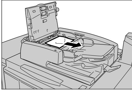
4. If there are instructions to turn the wheel, turn the green wheel to eject the document upward.
