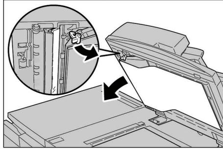
Part of the document cover pulls away from the assembly which allows better access to the second-side scanning lens assembly.
