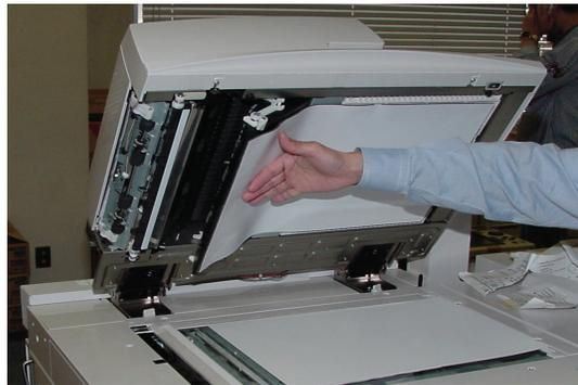
5. Wipe the mirrored glass, metal strip, **both** sides of the white-plastic strip, and the rollers with a soft cloth moistened with water to remove any dirt, and then wipe it with a soft, dry cloth.
