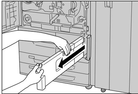
5. Hold the used waste toner container firmly with both hands and put it into the provided plastic bag.
