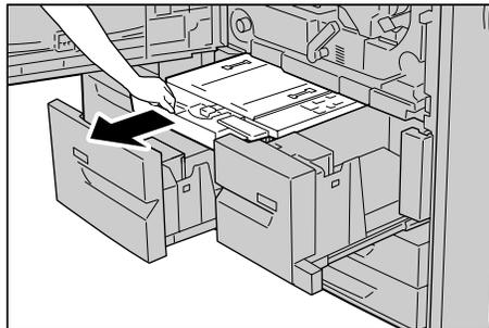
4. Lift up the lever 4a and then remove the jammed paper.
