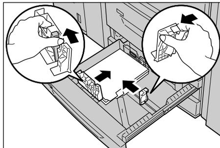
Ensure that the levers are positioned correctly.
