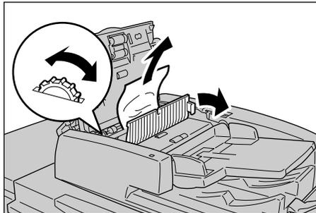
6. Turn the green wheel to eject the document upward.
