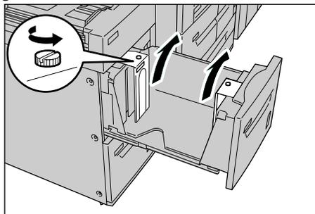
4. Attach the guides according to the hole of the paper size to change, and tighten the screws.
