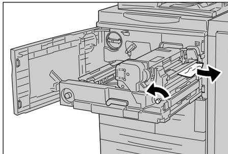
7. Shift the lever 3b on the right of the fuser unit as necessary and then remove the jammed paper.
