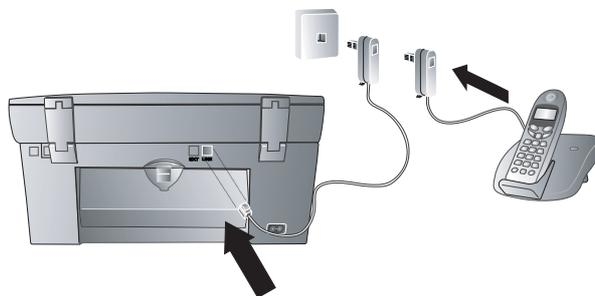
You can connect additional devices to separate sockets on the same line even if they are in different rooms.
