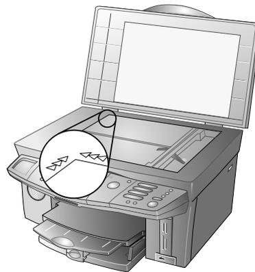
If you would like to copy a detail (such as a graphic) of your document, position the document such that the corner of the detail is up against the origin. Using the zoom function, you can separate the desired area from rest of the document.
