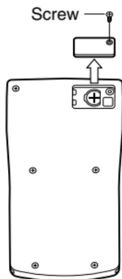
4. Wipe a new battery with a dry cloth, and then load it into the calculator with its positive ⊕ side facing upwards (so you can see it).
