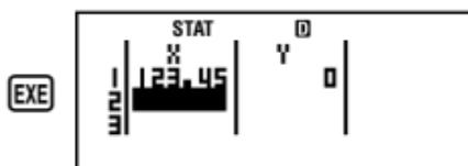
Registering a value causes the cursor to move down one cell.
